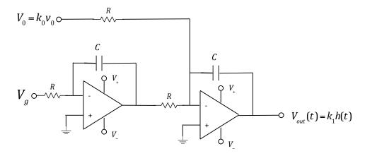
$V_0$  is fixed at  $V_0 = k_0 v_0$ , where  $v_0$  is the initial upward velocity. All  $R_0$  are equal and all  $C_0$  are equal. Assume all capacitors are initially discharged.
