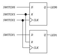
When SWITCH2 goes HI, the state of SWITCH0 and SWITCH1 will be loaded to LED0 and LED1. SWITCH3 will *asynchronously* turn those LEDs off as soon as it goes HI. Recall that in class, we gave an example of a simple data latch as shown below:
